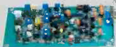
EN-10 Designed to work with graphics boards outputting analog RGB. Requires external sync generator.
