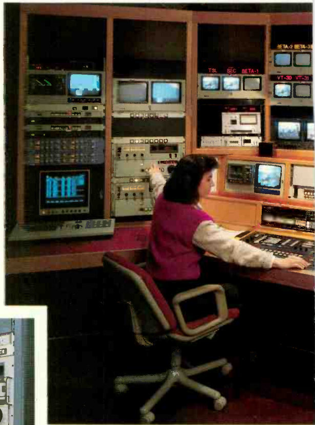
Master control switcher works together with the distribution switcher and machine control.
