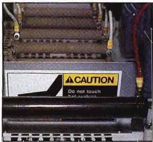
An overheated power resistor often will point to the cause of a power supply fault.
