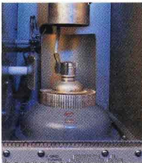
EIMAC's 5CX1500B broadcasting tube in KGLT radio station's transmitter.
