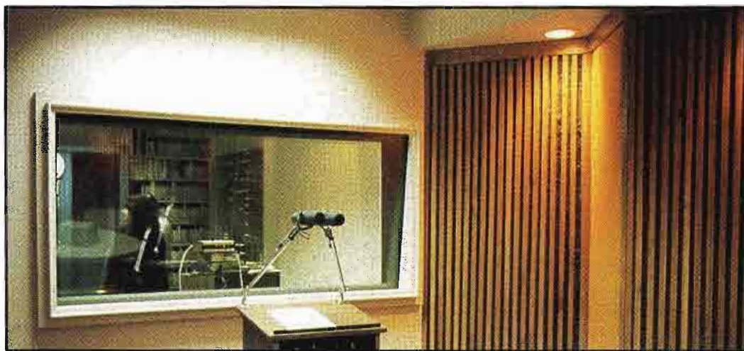
Using a wall washer fixture may prevent glare from large windows while providing even room illumination.
