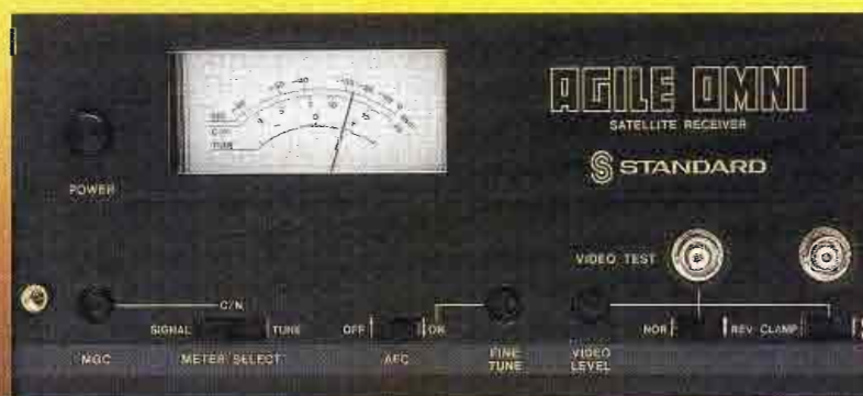
Operating functions including MGC, AGC, AFC, level sets, normal/invert video, clamp/unclamp video, skew, subcarrier frequency selection, video and IF test points are conveniently located on the front panel. Meter reads C/N ratio, signal strength or center-tune.
