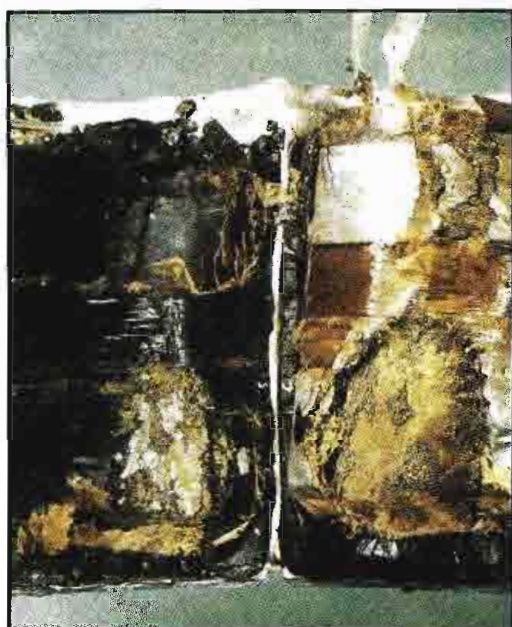
Figure 23. Internal view of an aluminum electrolytic capacitor that failed because of anodic corrosion. (Reference 29.)
