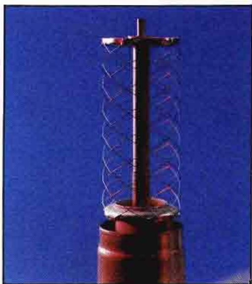
The useful operational lifetime of a power tube is determined by the filament structure, shown here. The mesh construction of this filament provides a rugged structure that is resistant to shock and vibration.
