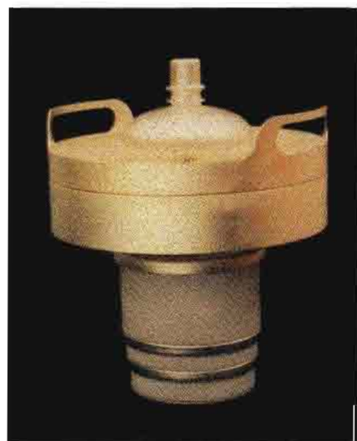
Figure 13. A new, unused 4CX15,000A tube. Contrast the appearance of this device with the tubes that follow.
