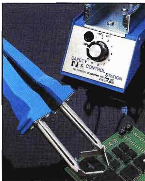
The control station, shown in the background, allows the probe tip temperature to be carefully controlled to prevent damage to the ICs.
