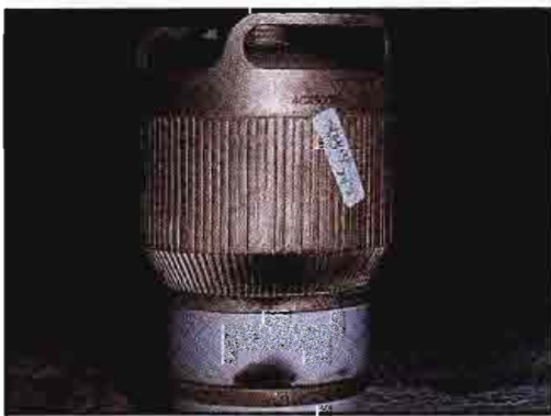
Figure 16. A 4CX5,000A tube that appears to have suffered socketing problems.
