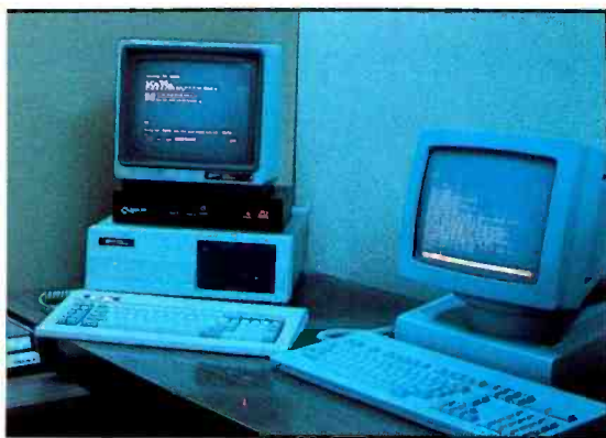
The center computer acts as the master controller for the local area network (LAN) system. The terminal on the right can be used to prepare messages and other distributed tasks.
