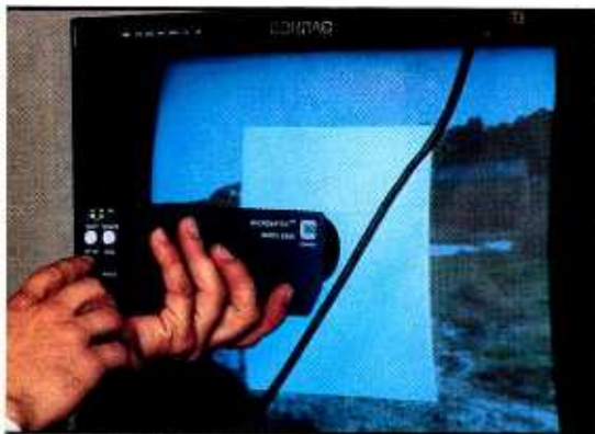
The photometer is placed against the center of the CRT during the measurement period. The alignment typically takes less than a minute.
