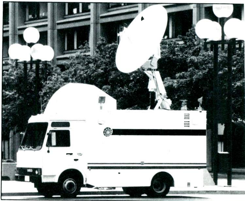
A 2.4-meter uplink truck with a roof-mounted antenna.
