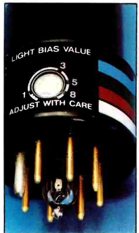
Bias lighting to reduce lag may be adjusted through an in-base control on some tubes.
