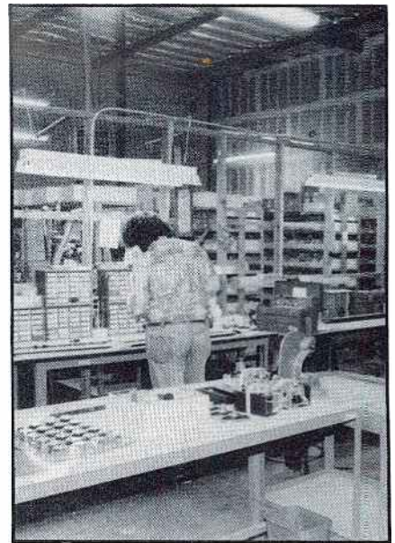
Adjacent to the electronic assembly area is a mechanical assembly section, where mechanical components are fitted together and circuit boards are installed in larger systems.
