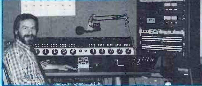
Typical installations of Ramko Research audio equipment. Shown are a DC38-8S 8-channel stereo audio control board (top left), a bank of ARA-1612 audio routing switchers (top right) and a DC38-10 10-channel mono audio control board.
