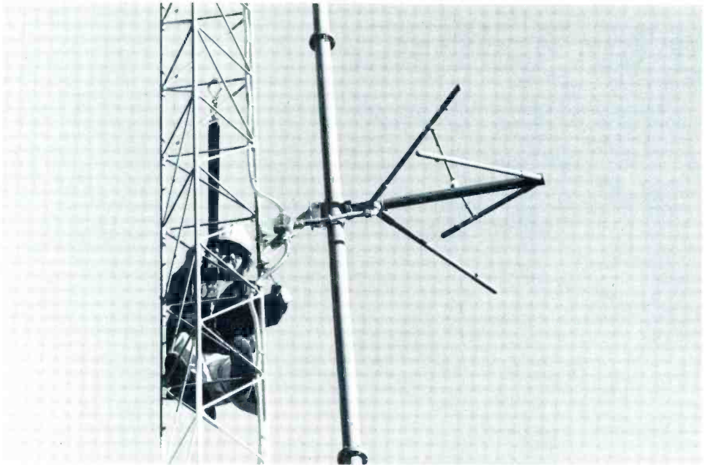
A JSCP FM antenna undergoes final testing and adjustment at the field measurement range.
