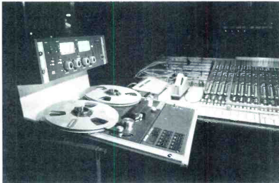
The A-810 shown is installed in one of Editel's studios. The machine (here in the console configuration) also is available in portable and rack-mount models.
