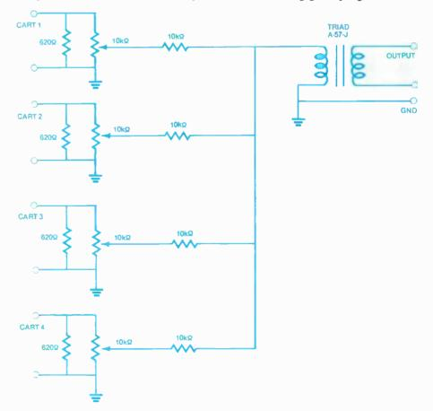
Figure 10. Simple submixer for inputs of a similar nature.
