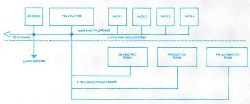
Figure 1. Grounding system layout for radio station with local transmitter.
