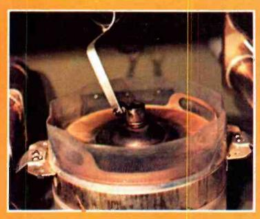
(a) Just before modification. Note discoloration of tube, which had less than 2000 hours on it.
