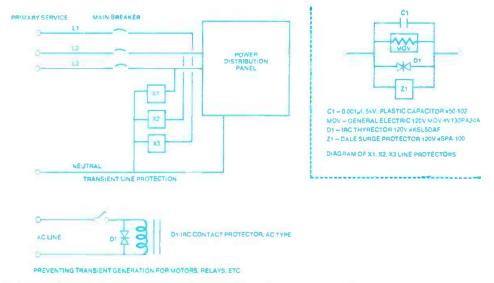
Figure 3. Methods of suppressing transients on the ac power line.
