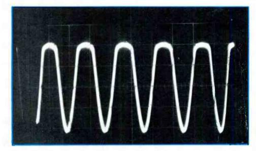
Figure 12. A clipped waveform that can be used to check for proper system phasing.
