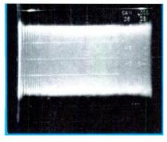
Figure 5(a). Sweep pattern with correct equal zation.
