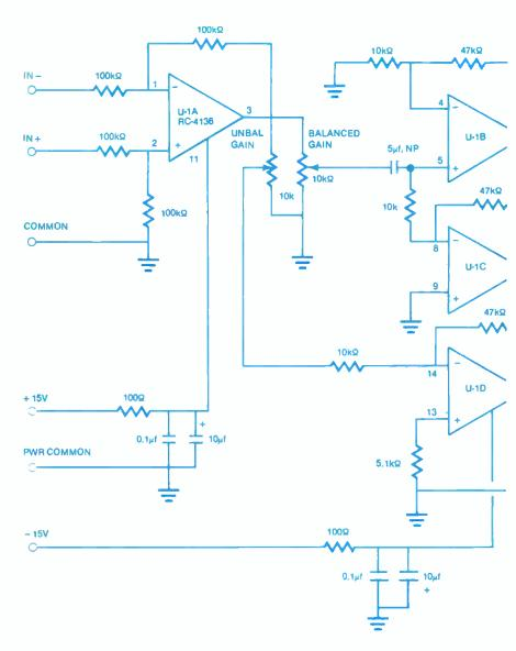
Figure 9. Buffer distribution amplifier.
