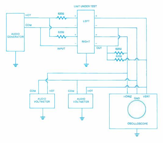
Figure 4. Tape deck alignment test setup.
