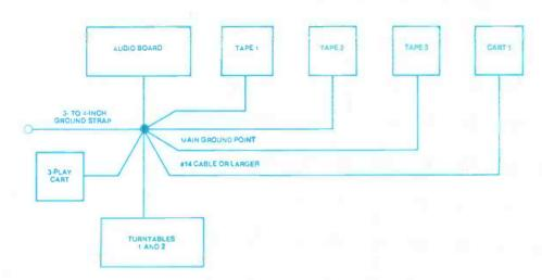
Figure 2. Ground system layout for individual equipment rooms.
