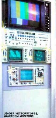
LEADER VECTORSCOPES, WAVEFORM MONITORS, SYNC/TEST GENERATORS AND OSCILLOSCOPES PHOTOGRAPHED AT REEVES TELETAPE, NEW YORK CITY.
