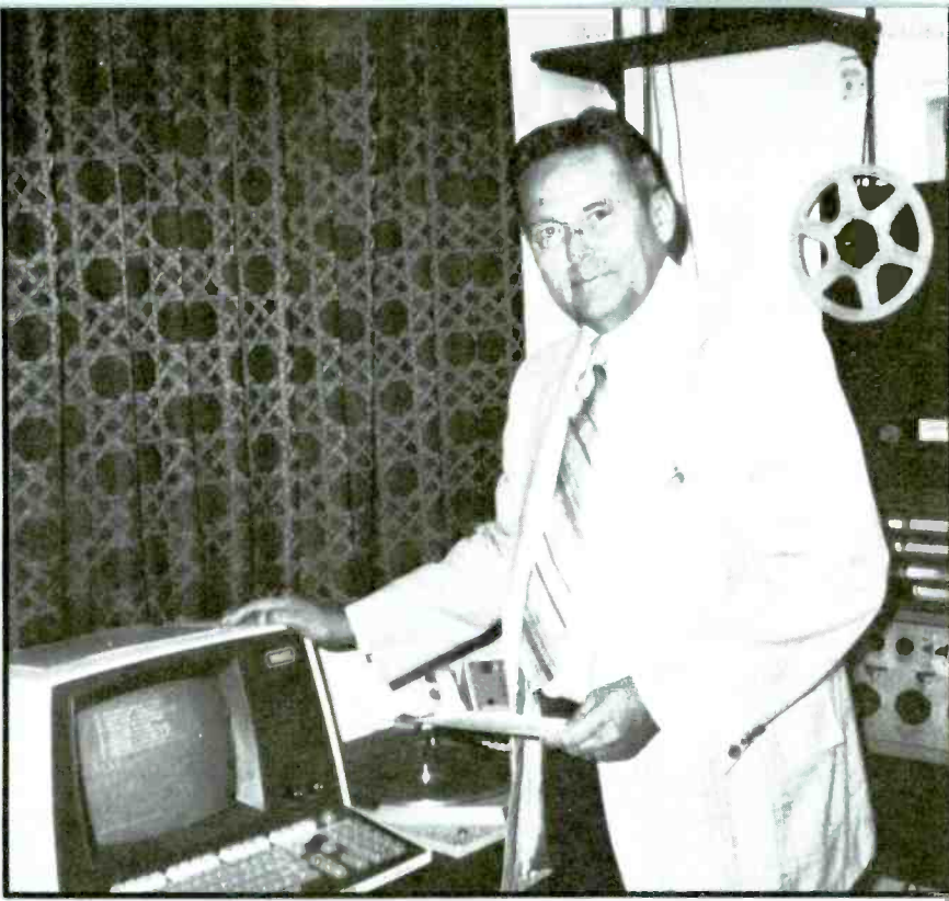
Kent Jones, station owner, demonstrates use of the Broadcast System terminal located in the control room. This terminal is used to place identification information on carts, as well as for other program automation functions. In all, the station uses three terminals for accounting functions and program automation control purposes.
