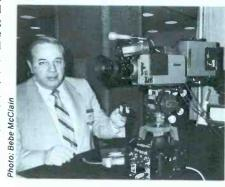
Philip Godfrey of ABC Engineering inspects the Frezzolini system that provides an interface for attaching a small JVC portable VHS recorder to any ENG camera.
