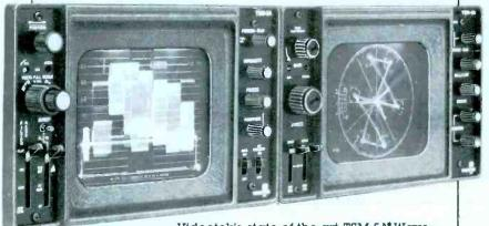
Videotek's state-of-the-art TSM-5A\* Waveform Monitor and VSM-5A\*Vectorscope reflect this on-going commitment, with such innovative features as Internal Graticule CRT for precise parallax-free signal analysis, and Non-Glare Shields to eliminate distracting ambient light. TSM-5A also includes selectable 1H mode for easy one-line viewing, and 0.5 µs/div. scan rate for the most accurate time-base measurements.
