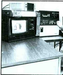
The author, with some of WNEV-TV's newly purchased equipment. Shown (left to right) are a video waveform monitor, a Panasonic AU-300 1/2-inch VCR, a Convergence ECS 103B editing console, a Panasonic AU-300, a Convergence SE-100 editing effects/switching system, an Ikegami HL-83 camera and a bolt-on Ikegami HM-100 M Format portable field recorder.
