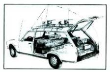
radios for program signals, as well as cabling, mics and mic stands. Larger vehicles are also available.
