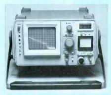
vides quantitative and calibrated measurements of high accuracy and reliability. Precision-calibrated loss and distance measurements are possible with this rugged, portable instrument. A chart recorder for documentation complements the CRT display for measurements on multimode 125μm OD fibers with a core diameter of 50µm.
