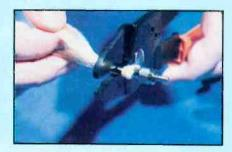
Fiber-optic connector being attached to a fiber cable using Kevlar as a strain relief beneath the crimp sleeve.
