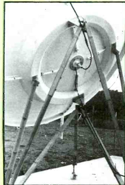
Antenna polar-mounting arrangement.
