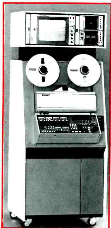
Ampex was one of the exhibitors at IBC-'82 introducing new products. Shown here are the VPR-5 lightweight 1-inch helical-scan VTR (right), the ARC-10 integrated camera/VTR with supporting editing and control equipment (upper right) and the VPR-3 Type C 1-inch helical-scan VTR with companion TBC (above).
