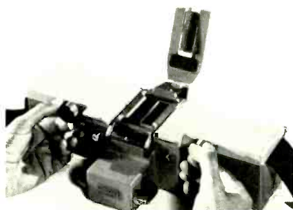
Ampex tape splicer in use.
