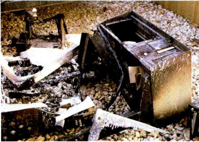
Remains of monitor bridge of AVR-2 Videotape Machine.
