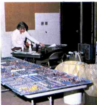
Printed circuit boards being washed. The solvent and water mixture was in the trash cans at the right of the picture.
