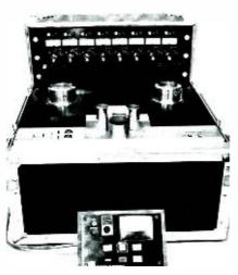
The complete Stephens line is modular in construction, and all subassemblies are easily removed for servicing. Each system's complexity has been reduced to a minimum and repairs can usually be undertaken by substituting a plug-in circuit board.
