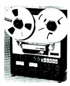
bilities to professional users at AM-FM radio and TV stations. It incorporates variable speed, 10<sup>1</sup>/<sub>2</sub>-inch reel capability, full remote controls and a built-in 4x2 mixer. The recorder has a 3-motor tape drive sytem with a capstan servo dc motor that provides greater torque with improved operational control and speed accuracy. A universal supply permits operation on ac power anywhere in the world.
