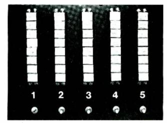
**Push-buttons** select the source to be chosen for each recorder (1 through 5 shown). Toggle switches at the bottom activate a clock system to automatically start the recorders.
