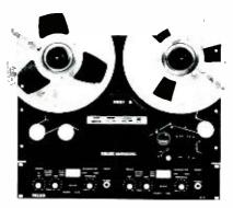
The 3000 is a heavy-duty commercial tape transport with Telex RP85 record/reproduce preamplifier. Tape transport accepts reels up to 10½ inches and includes automatic cycling, automatic cue release (AQR) and CMOS logic tape motion controls. The preamplifier has tape head connections that can accommodate all standard track and channel configurations offered in the 3000 tape transport series.
