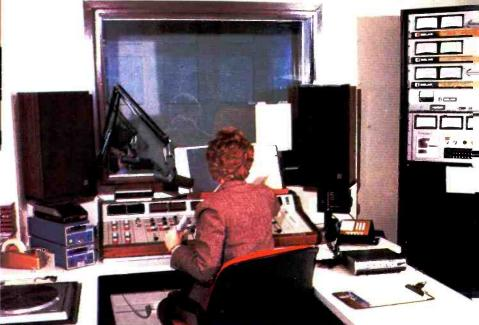
A view inside KBIA's main Studio A announce/control room, with staffer, Becky Preuss, at the controls. On the left are Technic SP-10 turntables and UMC Beaucart cartridge machines. The announcer faces and operates the Broadcast Audio System 16 audio console; Electro-Voice audio monitors flank the viewing window. On the right is an equipment rack housing the Belar monitors and Moseley transmitter remote controls.
