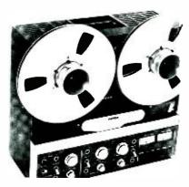
Universal reliable direct drive tape deck based on die-cast chassis; motion sensing and full logic control of all tape transport functions; two speeds; wide range available; for VU meters with peak indicators; professional headblock with 3-point mounting; electronics with high head room.
