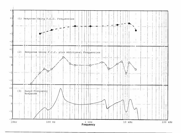
These frequency response curves illustrate the need for more measurement points than those required by the FCC proof. The curves are those of a hypothetical system, being checked from the playback of a cartridge machine to the input of one channel of a stereo FM transmitter (stereo generator).
