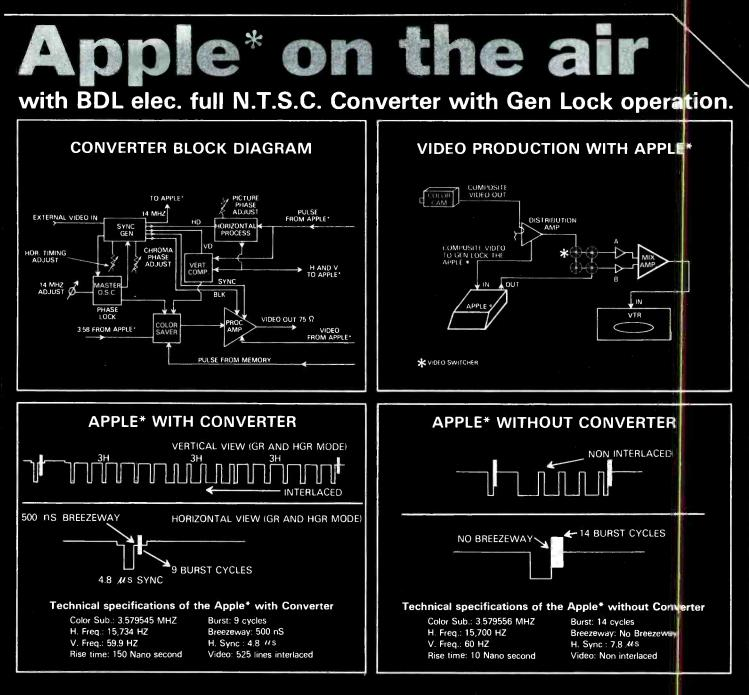
The converter process all horizontal and vertical impulses to give you a signal with 2 interlaced fields, and horizontal symp of 4.8 *us* with a (9) nine cycles burst flag place on the back porch at 500 nS of the horizontal sync trailing edge. The rise time as been corrected to 150 nS.
