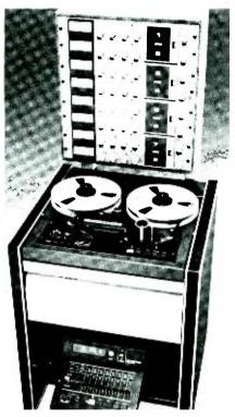
The MX-7800 ia a 1-inch 8-channel recorder featuring 30/15ips;  $600\Omega$ balanced output; dc capstan-servo system; console cabinet; automatic monitor switching; VU meters plus peak LEDs; constant tape tension with dynamic braking; dual-frequency test oscillator; lift-up access to transport; and punch-in/punch-out.
