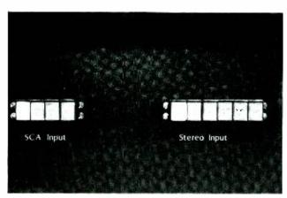
**KBIA broadcasts** a main channel and uses an SCA transmission as well. The passive switches shown here are used instead of patch panels to determine what goes into the main channel and what goes into the SCA.
