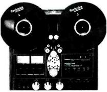
The 2-channel, 2-track, isolated loop, quartz-controlled tape deck design of the RS-1500US features increased dynamic range, lower noise and editing/splicing capabilities required in professional applications. Design considerations include low modulation noise; low head wear; stable high frequency; separate 3-position bias and EQ controls; record/playback format is 2-track, 2-channel; and can be mounted in 19-inch rack.
