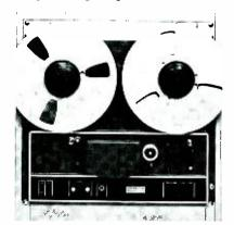
The 255 series of machines, developed for broadcasters, are compact 10.5-inch reel tape reproducers for mono or stereo automation or reproduce-only applications. This series has a heavy cast deckplate to maintain tape alignment, short headto-capstan distance to reduce flutter, trouble-free TTL logic, optional 25 Hz tone sensor for automation and optional remote control.
