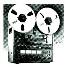
General features include compact <sup>1</sup>/<sub>4</sub>-inch 4-channel machine with dual speed (15/7 <sup>1</sup>/<sub>2</sub>-<sup>1</sup>/<sub>2</sub>ips) variable speed dc capstan servo, selective reproduce, motion sensing control logic, built-in test and cue oscillator, plug-in heads and easily accessible electronics adjustments.
