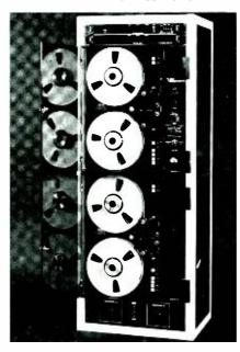
The Mark Twenty is a 20-channel professional communications logging system with extraordinary reliability, computer-style tape handling, directdrive dc servos, digital time indexing, "fail-safe" detecting and transferring circuitry; and all-digital remote controls.
