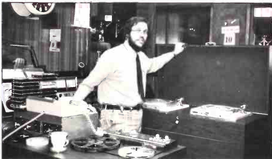
The control room turntables are protected by a hinged cover when they're not in use. (Most music at KPOW is on tape.) The turntables are mounted on their own sand-filled pedestals, which are isolated from other cabinetry to eliminate vibration and accidental bumps.
