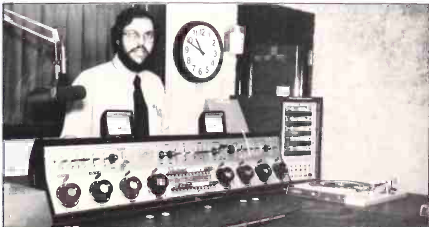
The production boards in both Studio A and B slide away from the wall for servicing from behind. The curtain on the window behind can be drawn back for visual cues to Studio C.
