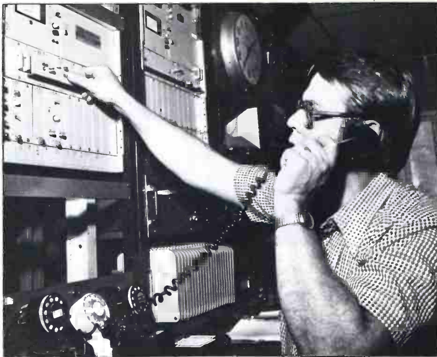
KOLN-TV engineer Lyle O. Kaufman exercises one of the many test and metering facilities of the station's new radio link. The GTE Lenkurt 78B3 transmitter shown here features built-in test facilities to perform such checks as deviation, power, output power, FM oscillator current, AGC level, crystal current and AFC without interrupting service.
