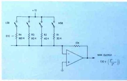
Figure 4 Simple D/A uses binary-weighted resistors.
