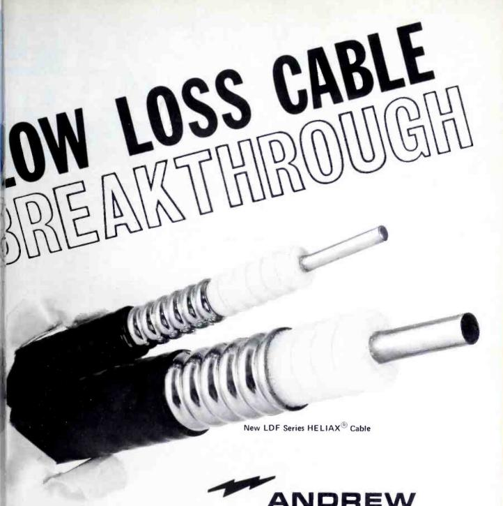
ower loss, improved moisture barrier, plus all ne traditional advantages of HELIAX foamielectric cable. New low density foam dielectric educes attenuation, almost to that of airielectric cables. Annular corrugations, in coninction with connector "O" ring seals, provide positive longitudinal moisture block.
