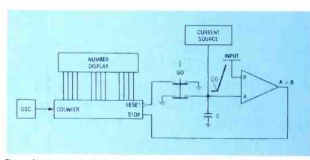
Figure 3 Indirect A/D digitizes the time needed to charge C to exceed input voltage.
