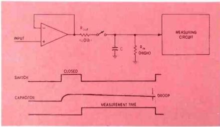
Figure 1 Basic Sampling Circuit.
