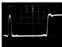
Figure 3 The same test signal applied to an enhancer clearly shows the noise reduction on the base line and improved K factor at the pulse edges.
