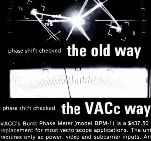
replacement for most vectorscope applications. The unit requires only ac power, video and subcarrier inputs. An easy-to-read analog meter indicates phase shift in the video burst relative to the subcarrier over a full 180 degree range with  $\frac{1}{2}$  degree accuracy. (360 degrees phase range can be obtained with a coax delay line).
