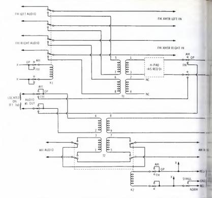
FM signal and when he hears the opening, he activates the COM-MAND switches (with the EBS FUNCTION switch in FM TEST, hopefully). The EBS cartridge for the FM station carries a 35 Hz tone at -18 db during the 25-second silent period to disable the automation "silent sensor".
