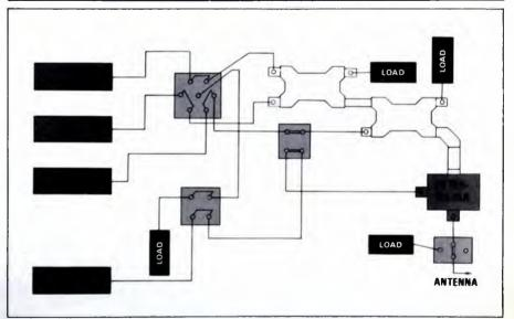
Four 55 kW vapor-cooled klystrons are used in the TTU-165c. A unique triplexing system developed for the WTAF-TV transmitting plant combines the outputs of three of the klystrons. As shown in the diagram, visual amplifiers 1
