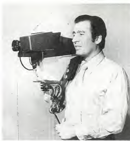
RCA's unique entry has a miniature viewfinder. Note the far-forward mainstructure positioning.
