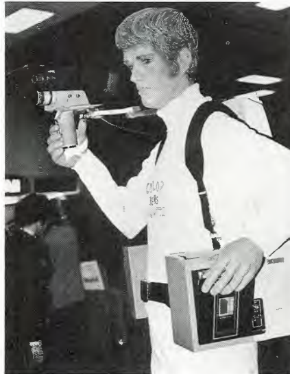
TeleAlpha's package includes the Akai camera and a modified cassette VTR. A separate edit console is included.
