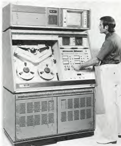
Here's the machine that has everyone guessing. It's the IVC 9000 two-inch broadcast quality helical VTR from International Video Corp.
