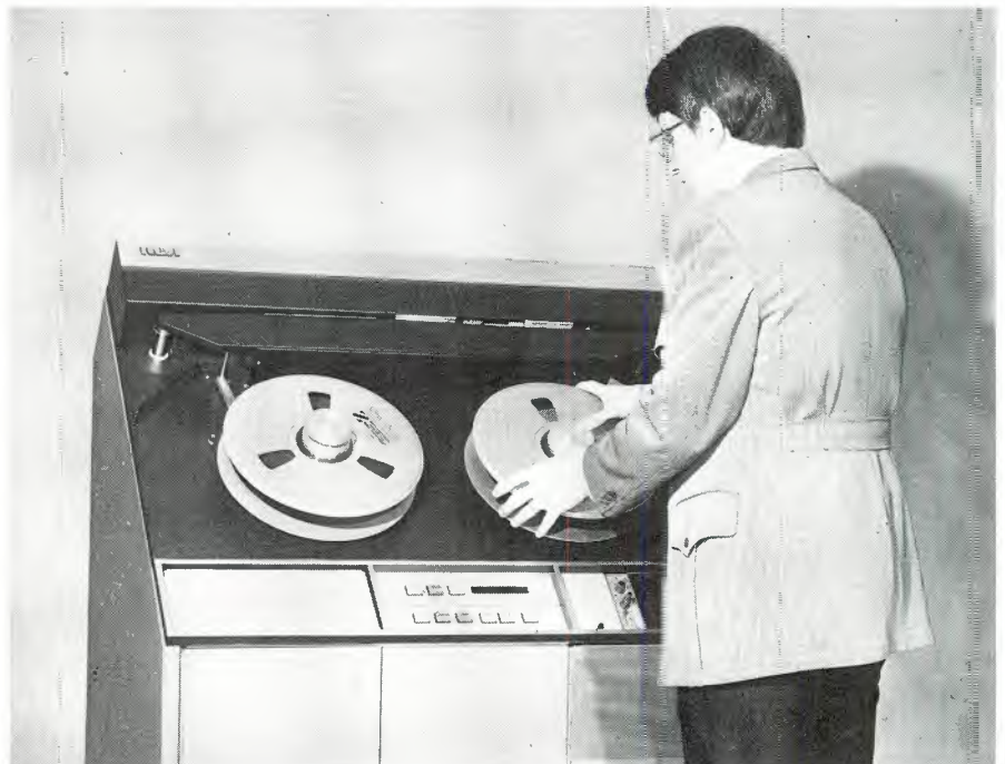
The RCA compact machine version introduced at NAB provides one-second lockup for stabilized color. It weighs in near 700 lbs.
