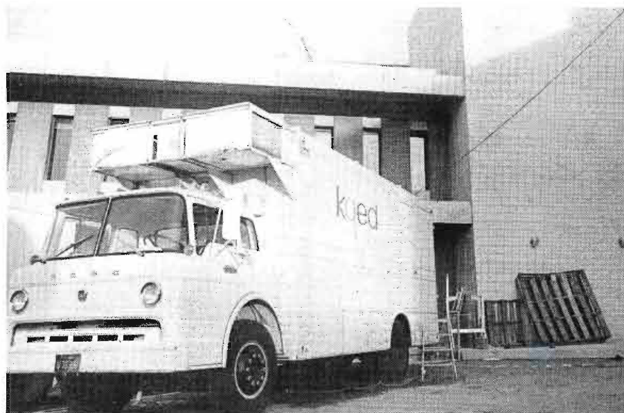
Two mobile vans housing three Mark VII color cameras and a VTR 2000 were used by KQED to cover the Pioneer 10-Jupiter encounter. Pacific Telephone used several microwave links to couple signals from Mission Control to various buildings at the AMES center and to the outside world. (Photo by Donna Roizen.)
