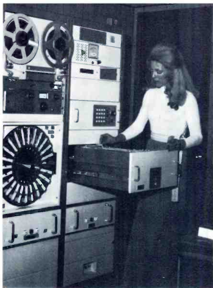
Fig. 4 Linda Shoblom programming the SMC 600 Digicard System. Each card represents an on-air event and can be changed easily any time up to the moment it is to be played.
