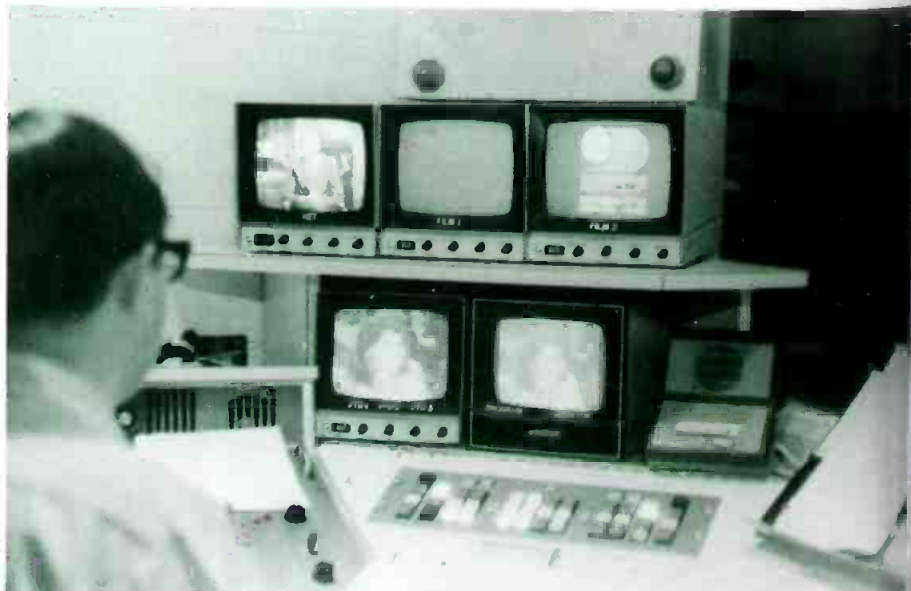
Fig. 1 At WESH-TV, the problem of lack of space for picture monitors was solved by the monitor-stretcher in operation here. See schematic in Figure 2.
