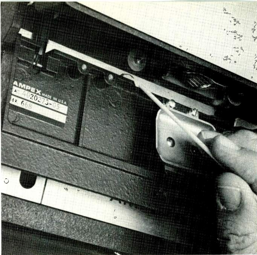
Fig. 2 Even the professional can improve his cleaning habits. This photo taken in a broadcast station shows bits of tape exactly where they were found. The swab stick points to a scrap uncomfortably close to the heads.
