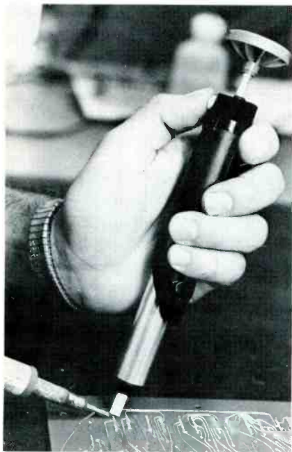
Fig. 5 Pneumatic device for removing solder.
