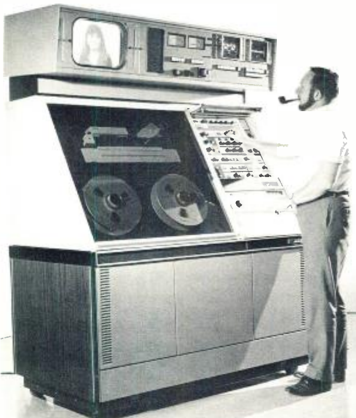
Fig. 1 The AVR-1 in operation. Note that operator makes operating adjustments near eye level. After the adjustments are made, the control panel cover can be pulled out and then down to cover the panel. Also, transport has a similar pull down cover.
