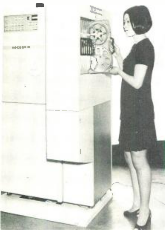
Fig. 1 The TC-701 cassette projector. Main projector controls are on the panel at the left. Cassettes are selected manually at the control panel or by an external computer programmer.
