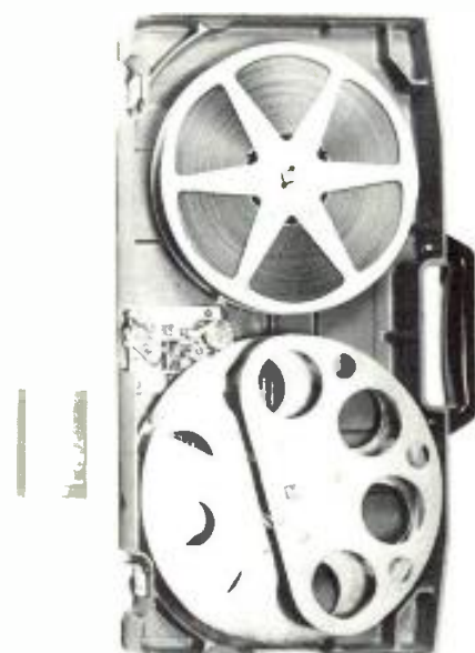
Fig. 4 Each cassette, as shown here, includes a 400 foot feed reel and a special take-up reel.
