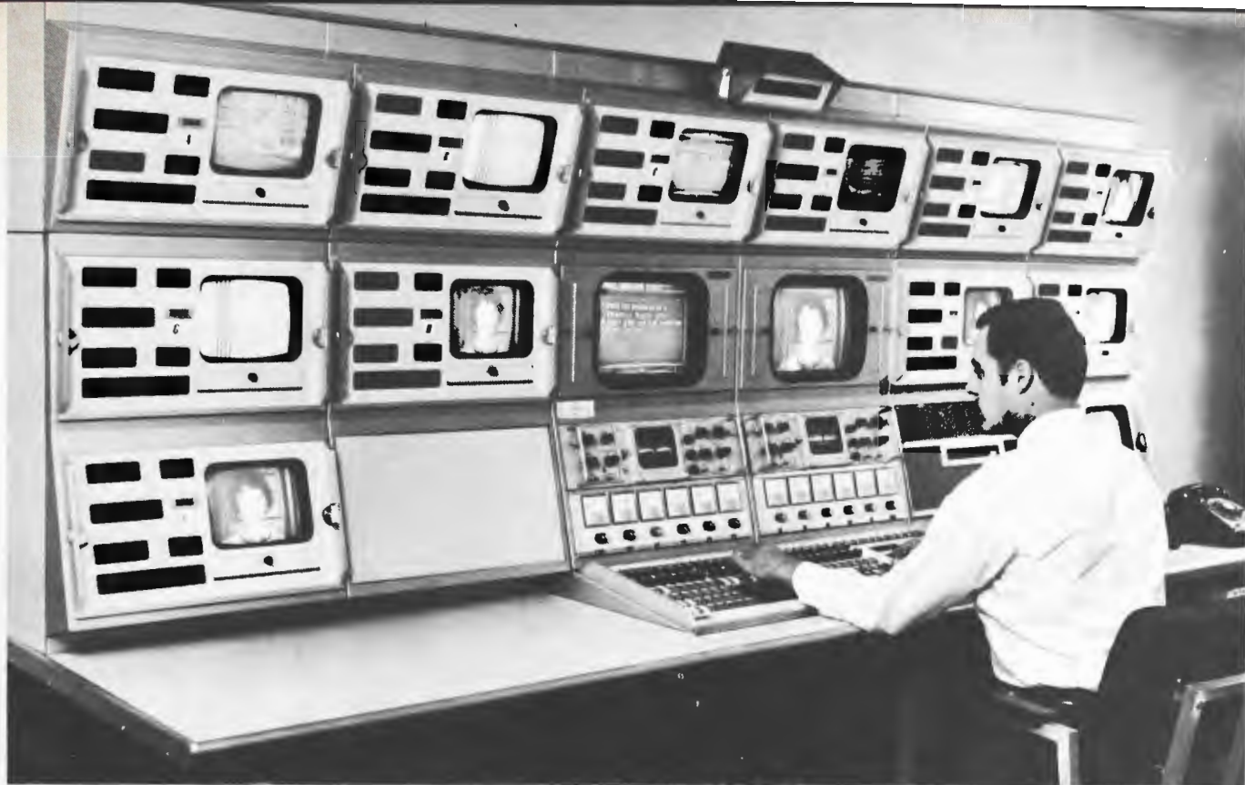
Fig. 1 Barely visible at the main console over the operator's left shoulder is a cartridge tape machine for emergency announcements. Note that five programs were being shown when the picture was taken.
