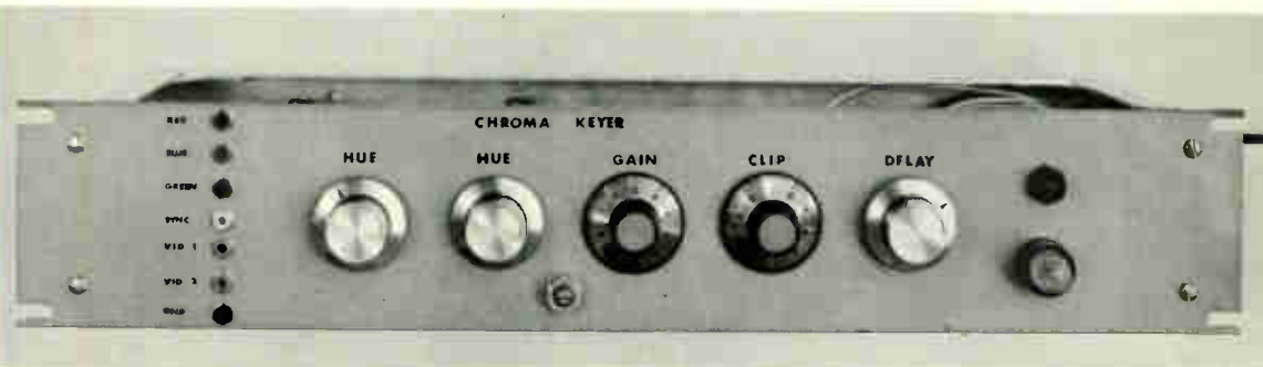
Fig. 2 Coarse hue control is at left, fine hue is second control from left. Balance adjust is between fine hue and gain controls.
