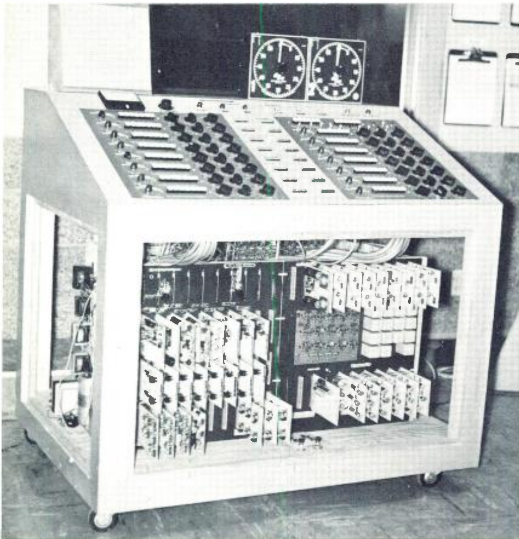
Panels removed from switcher control console, showing control logic (lower left), touch plate (center), and audio amplifier circuits at upper and lower right.
