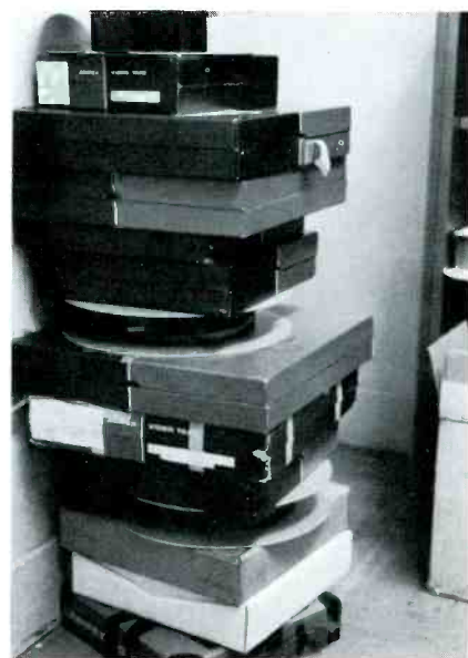
An example of how not to store magnetic tape. Stacking reels on top of others can bend the flanges and may damage the tape edges. Always store magnetic tape in boxes set on edge.
