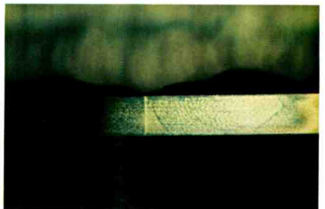
Fig. 4. Head tips exhibit blue-green and brown color. Coloration increases in density over 80 to 95% of the tip area. (Note appearance of Alfesil grain structure.)
