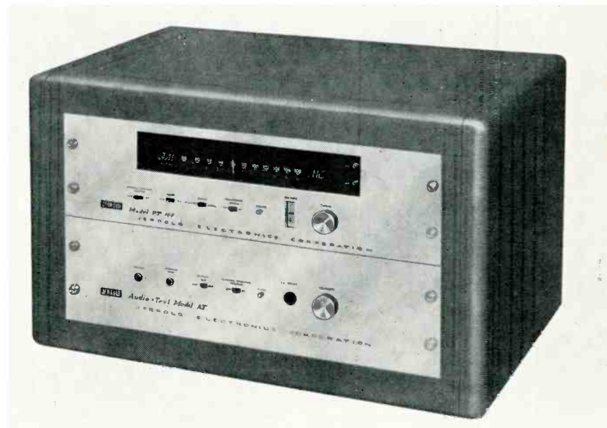
Fig. 4. FM can be inserted on a vacant TV channel using a unit similar to this.
