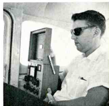
Fig. 5. Field-intensity meter in position.
