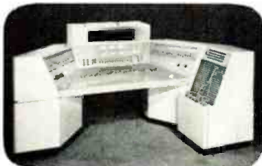
Custom-built Altec control console in ABC-TV's Studio One, New York. Note jack panel containing 720 connections that permit virtually any patching configuration.
