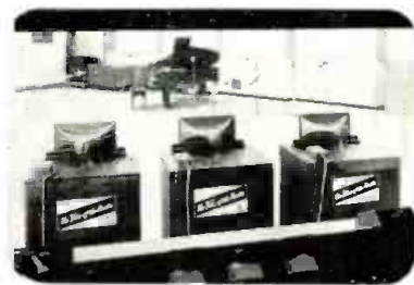
Control-room view of three A-7 Systems used for 3-channel PLAYBACK monitoring at United Recording Studios, Hollywood.
