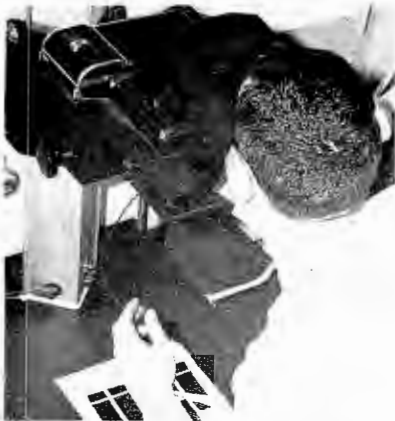
Fig. 3. Camera used to copy opaque.
