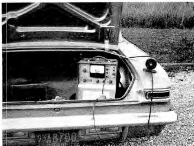
Fig. 1. Field intensity meter and antenna in operating position.
