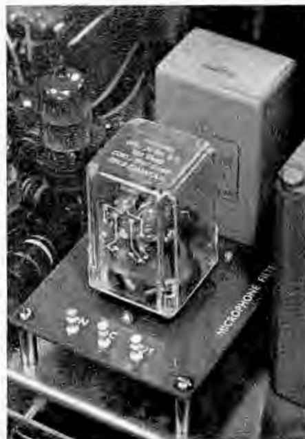
Fig. 3. Filter mounted in console chassis.
