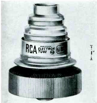
Fig. 1. 6181 beam-power transmitting tube, used as driver amplifier.
