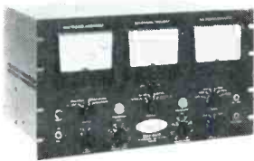
TBM-4000 McMartin FM/SCA MULTIPLEX MONITOR
