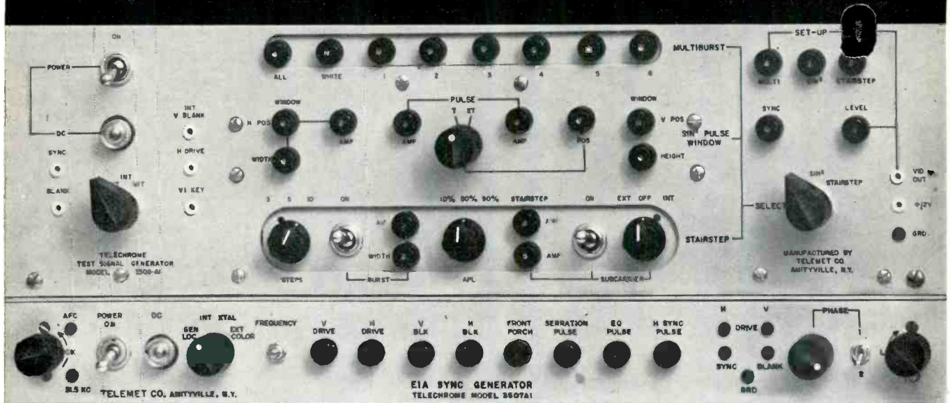
Model 3508A1 Video Transmission Test Set pictured with optional Model 3507A1 EIA Sync Generator
