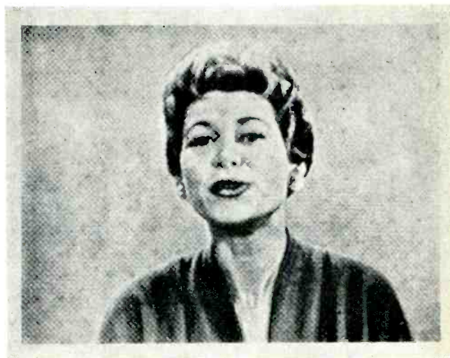
Figure 6. Picture from Strasburg television station converted by means of the Image-Orthicon. The 819 line picture was not spot wobbled.
