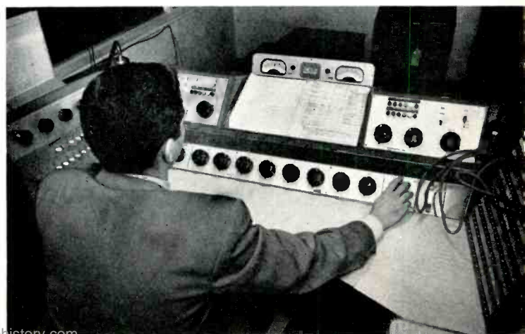
Figure 4. An audio control console modified for AGC. The meter to the left is the volume indicator, the one to the right is the gain-reduction meter. The gain-reduction meter was formerly a second volume indicator. It has been equipped with dual scales (VU and gain reduction) and can be quickly restored to its original volume indicating function in the emergency audio channel by operation of the small switch at its left. The other small switch to the right of the volume indicator serves to disable the automatic-gain-control when desired.
