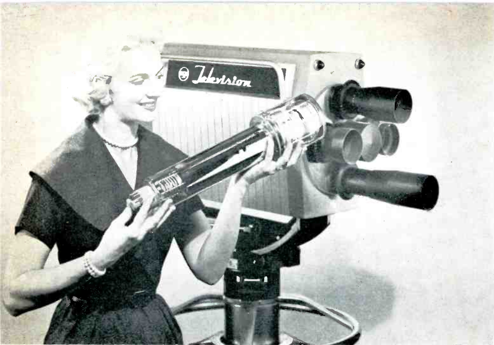
The 4 1/2-inch image orthicon tube displayed with new TK-12 RCA camera.
