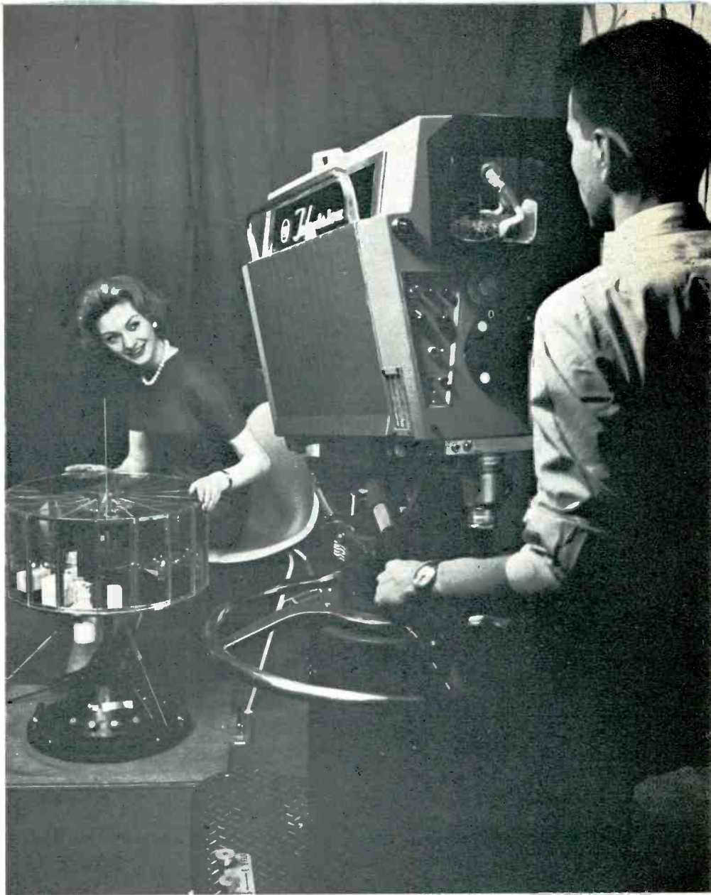
A half-sized model of the Tiros weather satellite is photographed with the new RCA camera which uses a 4 1/2-inch image orthicon tube.
