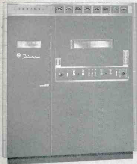
TT-2BL, 2-Kw Low-Band Transmitter
