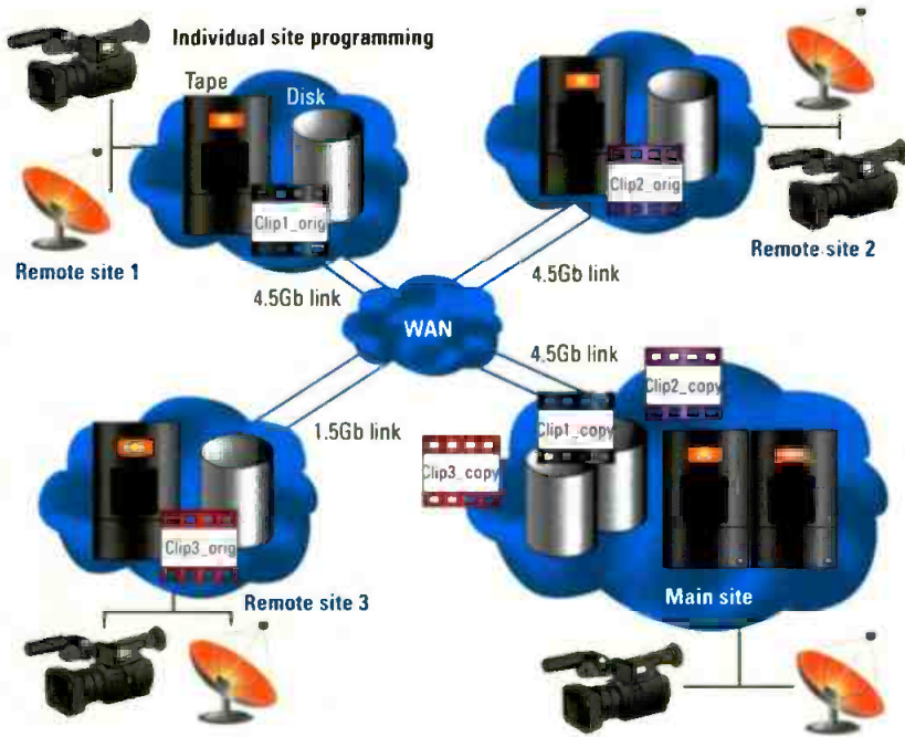
Figure 1. A private cloud archive provides standard archive functionality, as well as disaster-recovery facilities for multiple remote sites.
