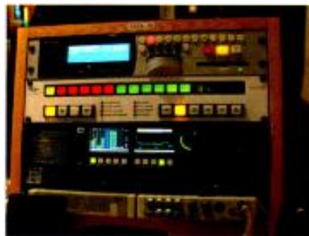
The PAM2 enables users to monitor surround sound and loudness for both incoming and outgoing streams.
