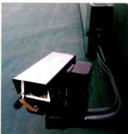
The centerfield cameras are mounted on Telemetrics PT-LWP-S3 pan/tilt heads that feature shot convergence technology and are enclosed in weatherproof housings.
