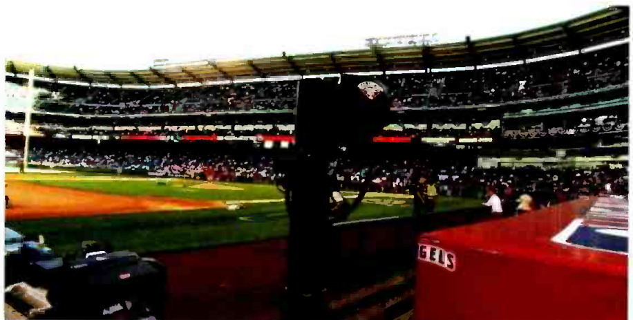
The dugout cameras, used for capturing field and stadium views, are each mounted to a Telemetrics Televator EP-S3 weatherproof elevating pedestal. Image courtesy MLB Network.
