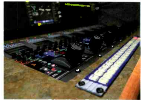
Shown here are the OCP panels for the Sony HXC-100 HD cameras, where shading and camera matching are completed prior to each production with a Sony BVM-L170 HD color grading monitor.
