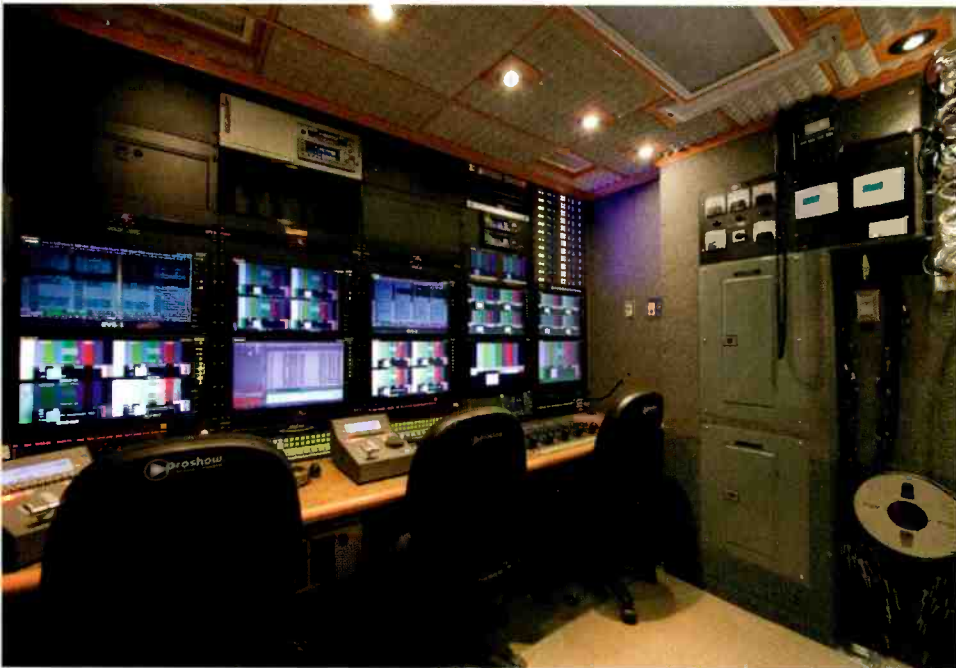
In the tape ops and Sony camera shading area, multiple feeds are iso recorded and archived for future storage by the client.
