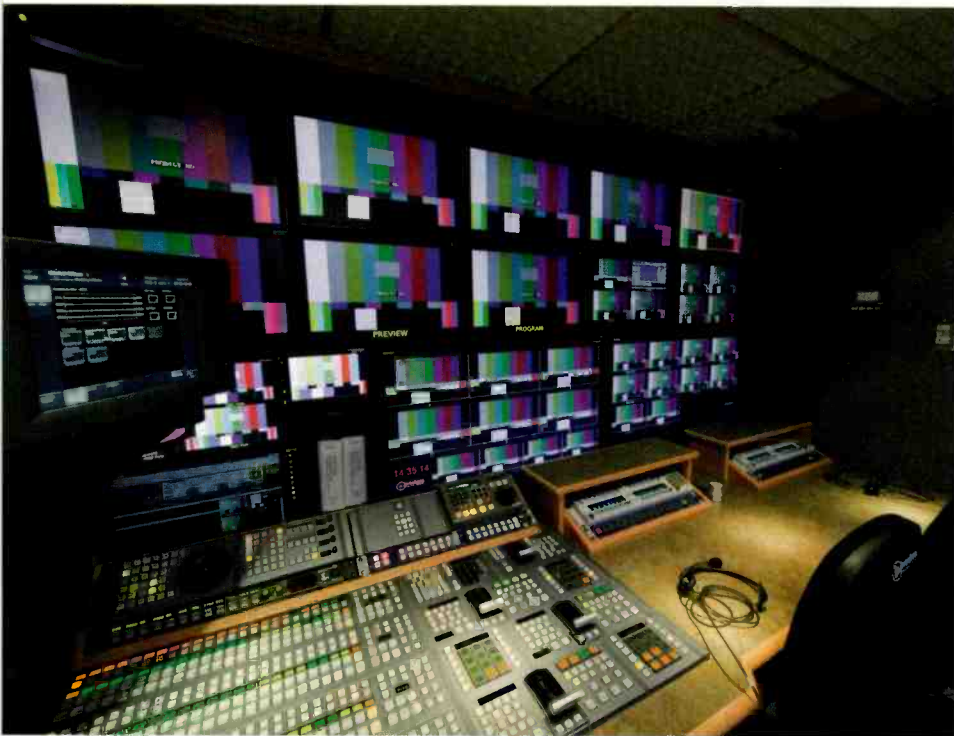
The main production area features a new Sony MVS 8000 GSF HD video switcher and reconfigurable monitor wall complete with Marshall displays running Miranda Kaleido-Alto multiviewer software.
