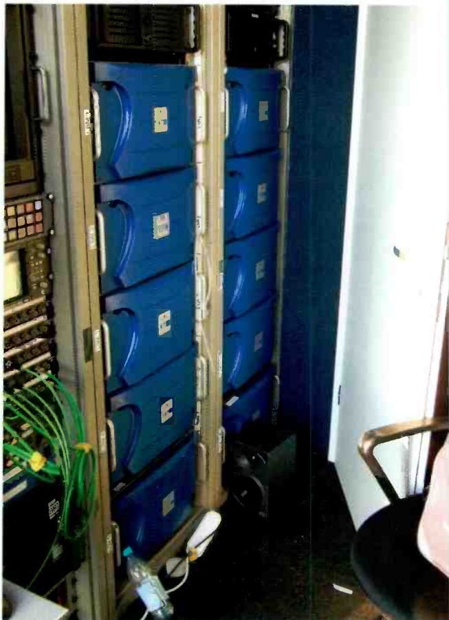
Shown here are EVS servers forming the original media server concept developed for the 2006 World Cup in Germany.
