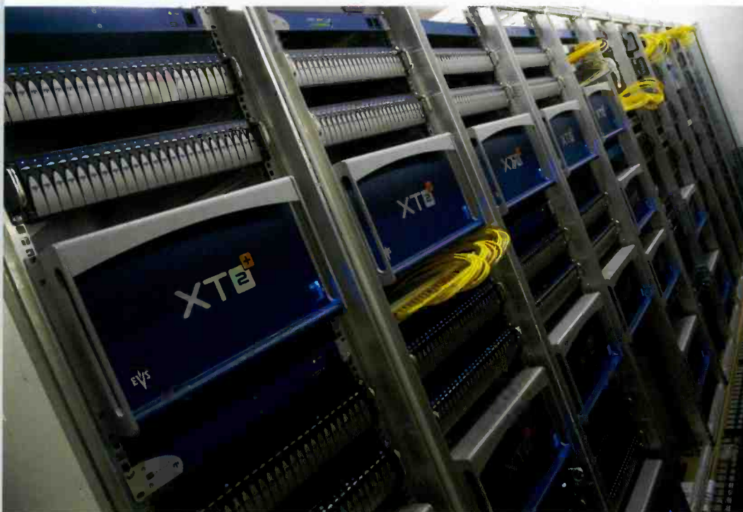
EVS is providing the host broadcaster, HBS, with HD multiple feed ingest and media exchange using a media server based on a network of XT[2] servers.
