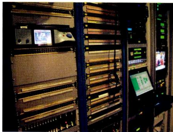
Vermont Public Television uses the Orban Optimod 8585 surround-sound processor to keep its viewers from having to constantly adjust the volume level.
