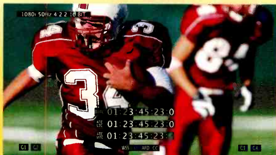
Image showing timecode and metadata overlay mode. G1-G4 indicate AES audio presence, WSS, VI, AFD and CC are present when highlighted.
