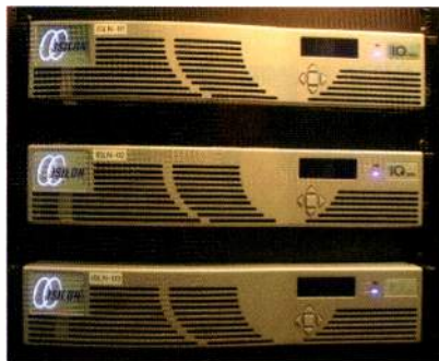
Students and teachers store their multimedia projects on a 9TB Isilon IQ X-series digital file storage system.
