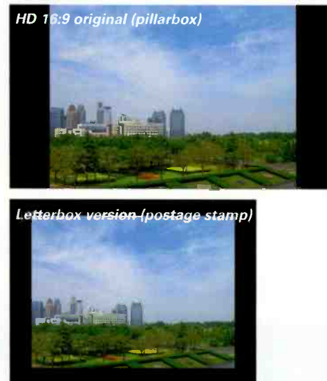
Figure 4. Example of adversely affected letterbox downconversion
