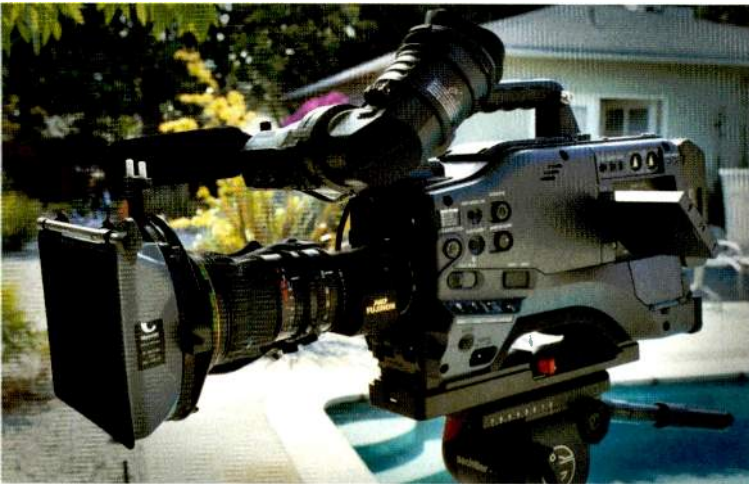
The HPX500 is a modestly priced 3-CCD camcorder that performs well in low light. The major reason: a 2/3in imager with resolution akin to the HVX200 but with concomitant larger pixels.
