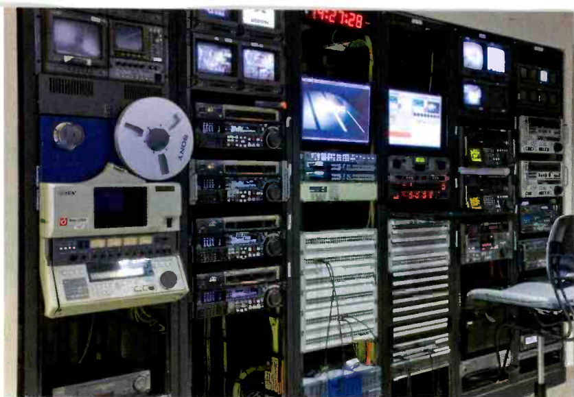
Game elements from around the country are collected in the feed/ingest area, which features support for a variety of formats, including a Sony 1in VTR (far left).
