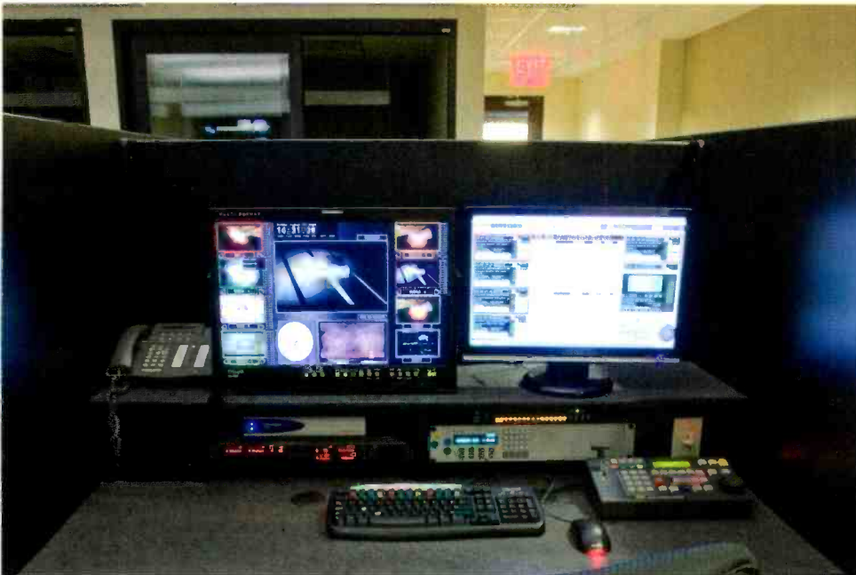
Game coverage and highlight reels are put together with the four Harris Velocity workstations. An additional six Velocity ESX software-only versions help develop pre-built packages and player profiles for insertion into the game coverage.
