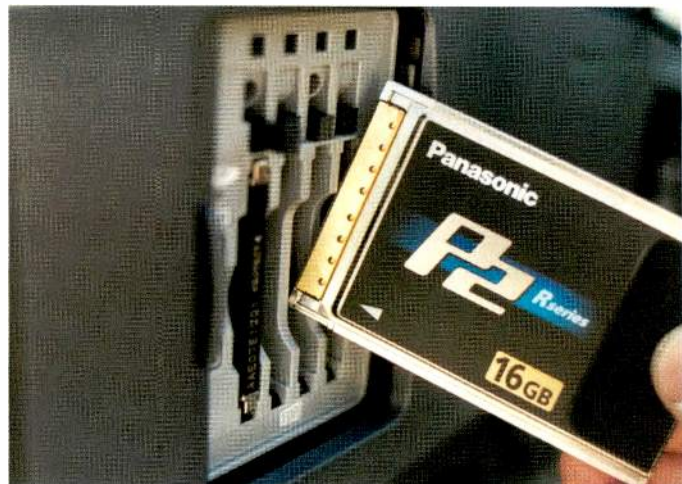
Outfitted with four 32GB cards, the HPX500 can shoot 320 minutes on a single load at 720p24 native mode.
