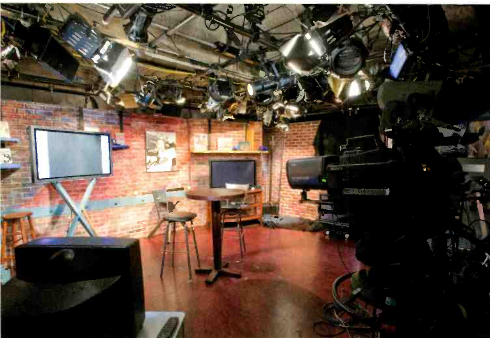
Each of three nearly identical production studios features two Sony HDC-1550 HD cameras with Canon 22x7.3 lenses and a small set that can be changed quickly when necessary.
