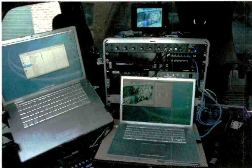
FOX News reporters have access to a Streambox encoder and related software linked to an Apple MacBook Pro laptop. A second MacBook Pro laptop is used for onboard editing and decoding.
