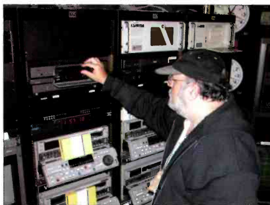
The audio and video capabilities of JVC's ProHD D-VHS tapes better suit WTTW-TV's needs than more expensive professional VTRs because the original ASI signal from the satellite is never decoded.
