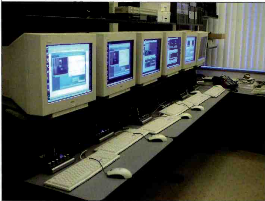
Each encoding workstation at X-Factor Communications has a mini audio mixer to fine tune audio before it goes to the encoders.
